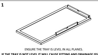
IF THE TRAY IS NOT LEVEL IT WILL CAUSE FITTING AND DRAINAGE ISSUES.
