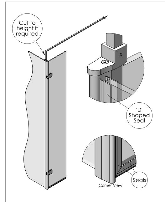
8. Fit 'D' shaped seal to hinge glass ensuring it seals on to the aluminium profile.
